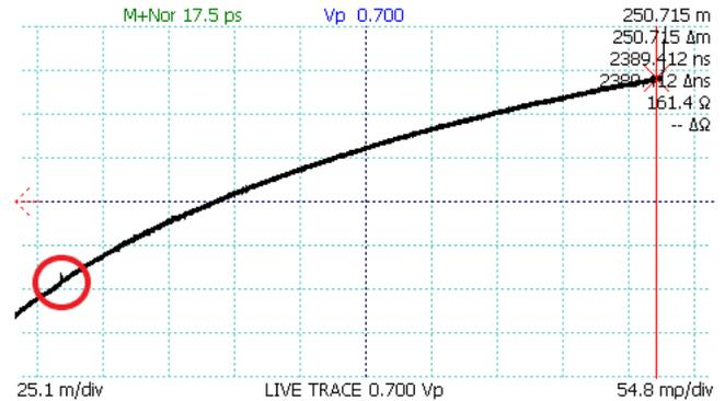
Figure 2: Small fault easily identified on a long cable.
