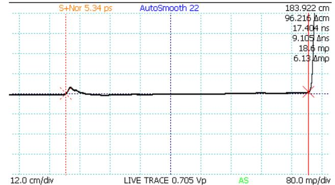
Figure 3: Measurement of distance between soft faults.
