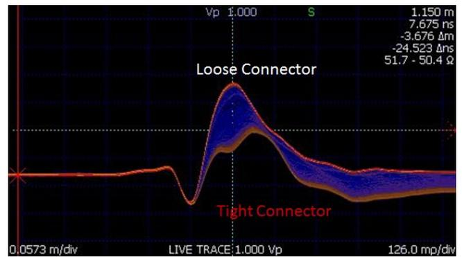
Figure 5: Intermittent fault detection with probability density plot.
